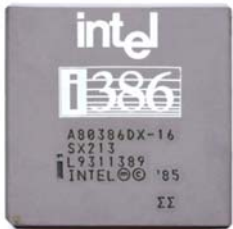
Intel 80386 DX rated at 16 MHz
