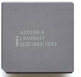
A 8MHz Intel 80286 Microprocessor
